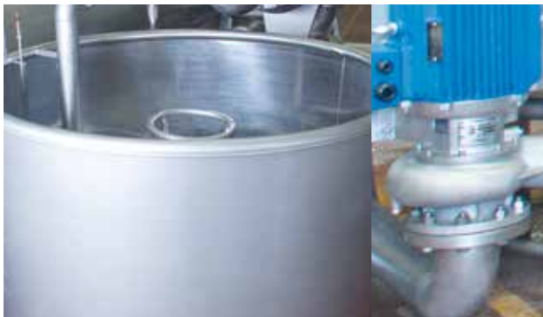
Service tank with feed pump, valves and stirring function
