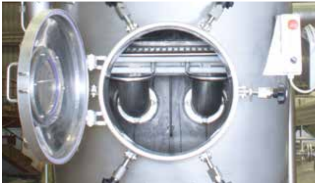
Service door and double guide ring
