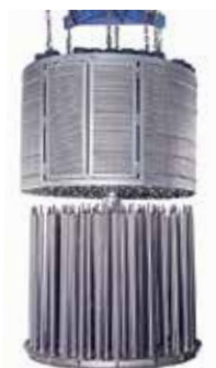
Step 3. Unloading basket is completely removed from carrier
